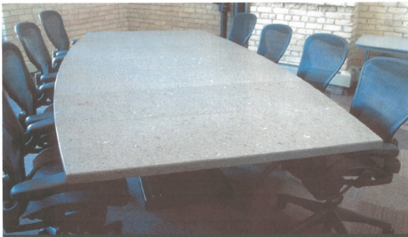
PAPER TABLE: Stanley Shetka, a professor of art at Gustavus Adolphus College in St. Peter, Minn., fashions countertops, doors, decorative frames, even walls and roofs from ShetkaStone, the material he makes from recycled paper.
